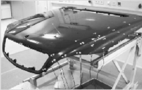
Figure 9: Measuring the irradiance eight-channel meter
