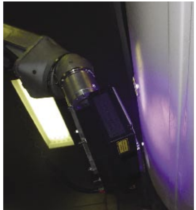
UV LEDs developed by Phoseon Technology use electrodes or microwave energy to excite mercury atoms that emit UV light in the process [picture courtesy of P Mills/UV robotics]
